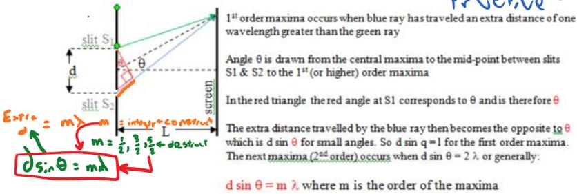
A diffraction grating is a series of lines usually several hundred lines per millimeter. Many sources, better constructive interference at high  $m$  AND better destructive between maxima. Also changes spacing of maxima.
