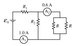
9. The figure above shows a circuit containing four resistors, a battery, and two ammeters. The current in ammeter  $A_1$  is 1.0 A, and the current in ammeter  $A_2$  is 0.6 A. The two resistors labeled *R* are identical. What are the currents in  $R_2$  and in each of the two resistors labeled *R*?
