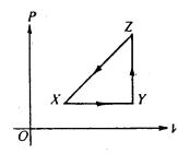
A thermodynamic system is taken from an initial state X along the path XYZX as shown in the PV-diagram above.
