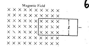
29. The figure above shows a rectangular loop of wire of width  $\ell$  and resistance R. One end of the loop is in a uniform magnetic field of strength B at right angles to the plane of the loop. The loop is pulled to the right at a constant speed  $\nu$ . What are the magnitude and direction of the induced current in the loop?
